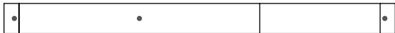
12' Run: 8' (243.84cm) Master Module, 4' (121.92cm) Slave Module, Dual Sensor End Set, and Intermediate Cable Assembly.
